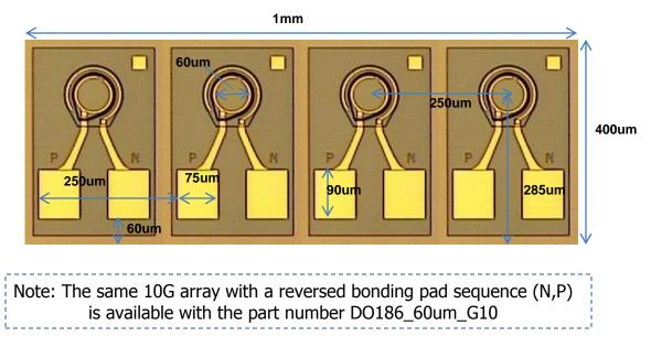
Attention: GaAs material and electrostatic sensitive device, observe precaution for handling.
